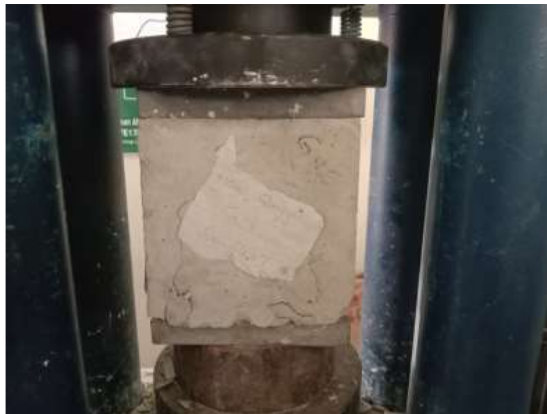
Figure 1. compression test according to ASTM (BS EN 12390-3)
