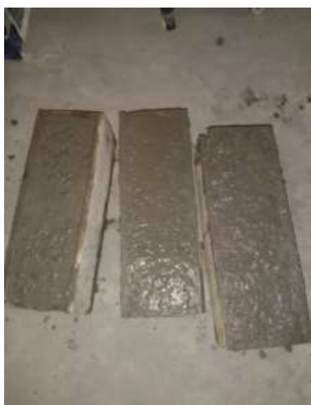
Figure 4. Flexural Strength of Beams (ASTM C 78 )
