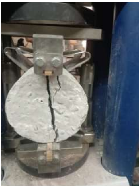
Figure 2. Splitting Tensile Strength Test of Specimens (ASTM C496)
